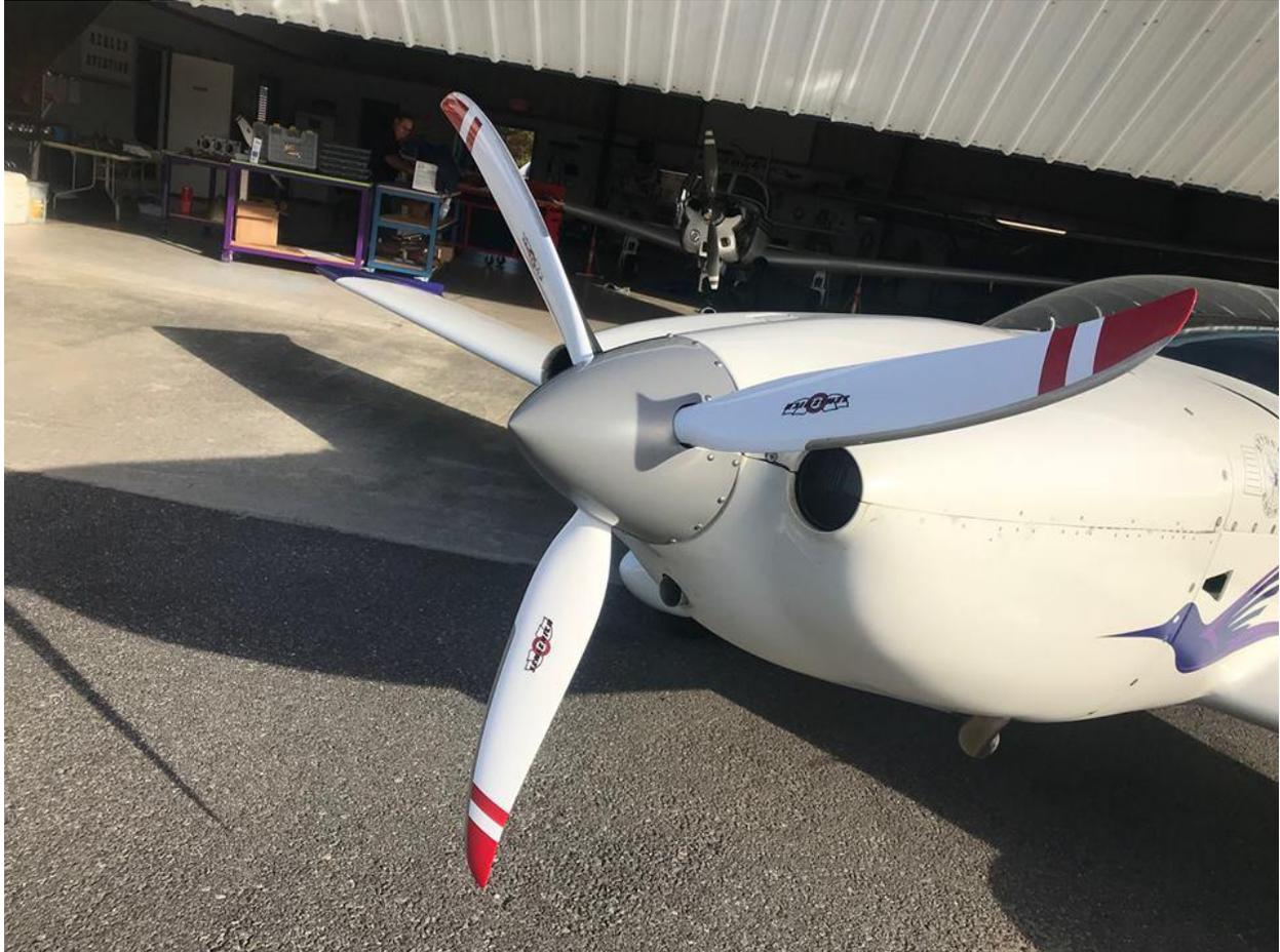
Third Test Prop: Sensenich (see a trend here..) 3 blade composite - hollow core - ground adjustable 58" prop.
